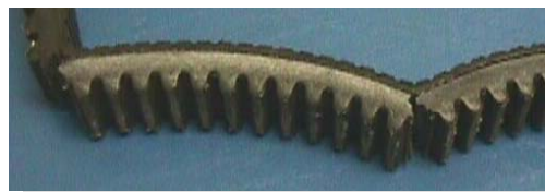
Flex cracks between cogs
