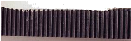
Uneven belt wear on one side only
