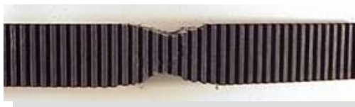
Concave top belt surface worn belt side
