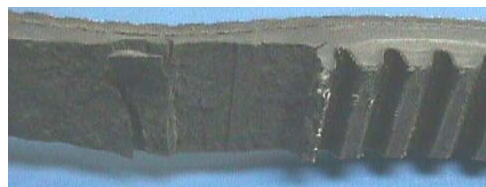
Sheared cogs, compression section fractured or torn
